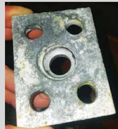
Close up view of the chainplate's aluminium backing plate
